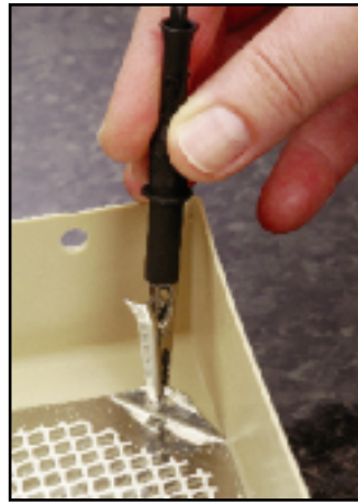
2a. ATTACH LEADS TO ELECTRODES USING CROCODILE CLIPS. 2b.
